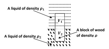
A block of wood of density  $\rho$  floats in an interface between immiscible liquids of densities  $\rho_1$  and  $\rho_2$  as shown above. Show that the ratio of the volume **V**<sub>1</sub> : **V**<sub>2</sub> of the block in the two liquids is given by;
