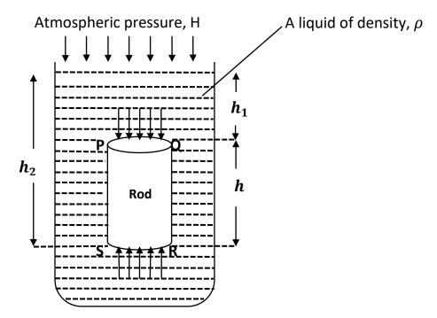
Consider a cylindrical rod PQRS of cross section area, A and height, h totally immersed in a liquid of density, p as shown above.
