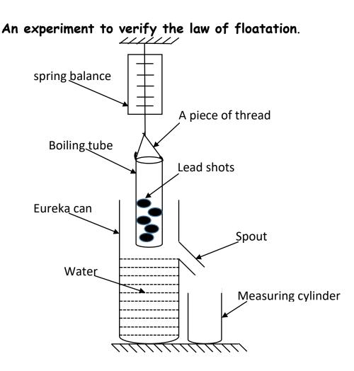
• Water is filled in a Eureka can up to the spout level, with a measuring
